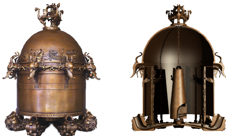
图4 新完成的张衡地动仪复原模型（左图），内部结构由“柱、关、道、机、丸”5部分组成（右图） Fig.4 New reconstructed model of Zhang Heng’s seismoscope. The interior structure consists of five parts including a general pillar, a trigger, eight roadbeds, levers and balls.
